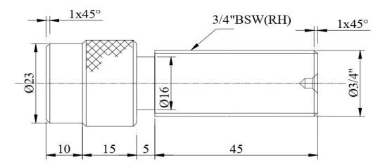
4. Prepare the specimen and make the Shaft and Bush as shown in figure using the Lathe.
