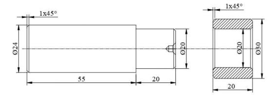
5. Prepare the specimen and make the Step turning & BSW and Metric Thread cutting as shown in figure using the Lathe.
