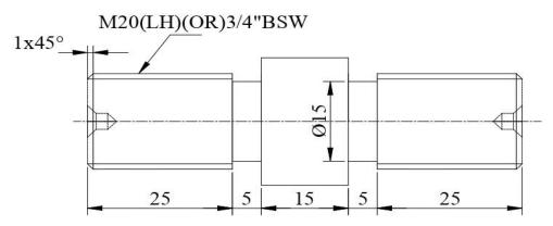
6. Prepare the specimen and make the Eccentric turning as shown in figure using the Lathe.
