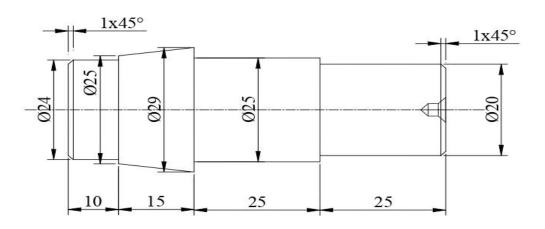
2. Prepare the specimen and make the Step turning & Knurling as shown in figure using the Lathe.
