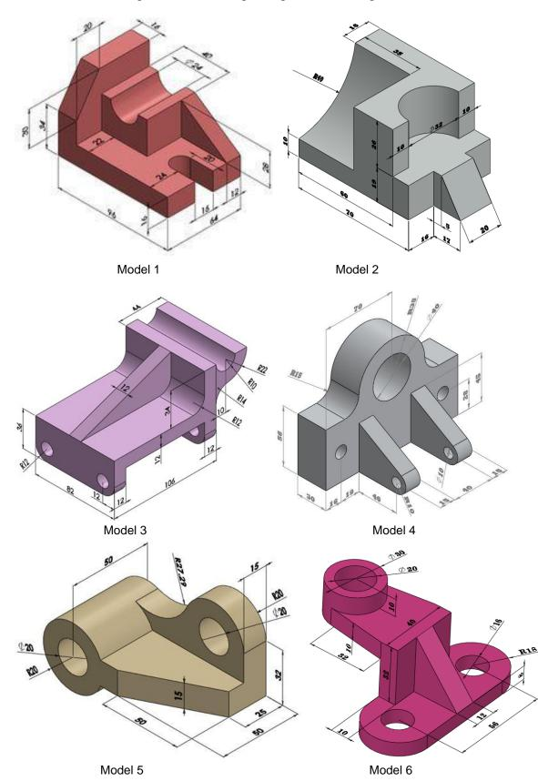
PART A: Draw the given 3D drawing using 3D modelling commands.
