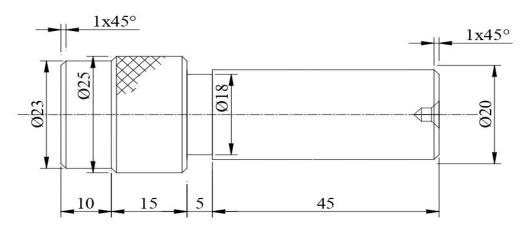
3. Prepare the specimen and make the Step turning &BSW Thread cutting as shown in figure using the Lathe.
