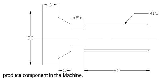
3. Using canned cycle - Create a part program for thread cutting, grooving and
